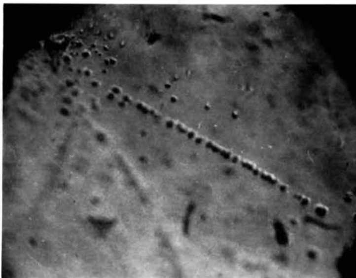
Fig. 6. A sub-boundary originating from a highly stressed region of the crystal surface (1090 \times ).
